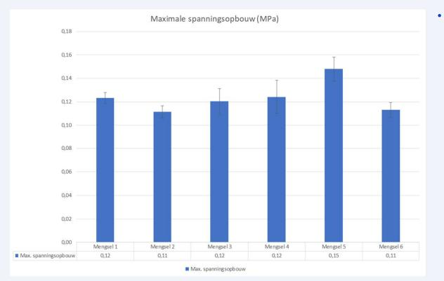
Maximum stress build-up (MPa) during TSRST for M1 to M6. The stress build-up per mixture is the average of three tests
